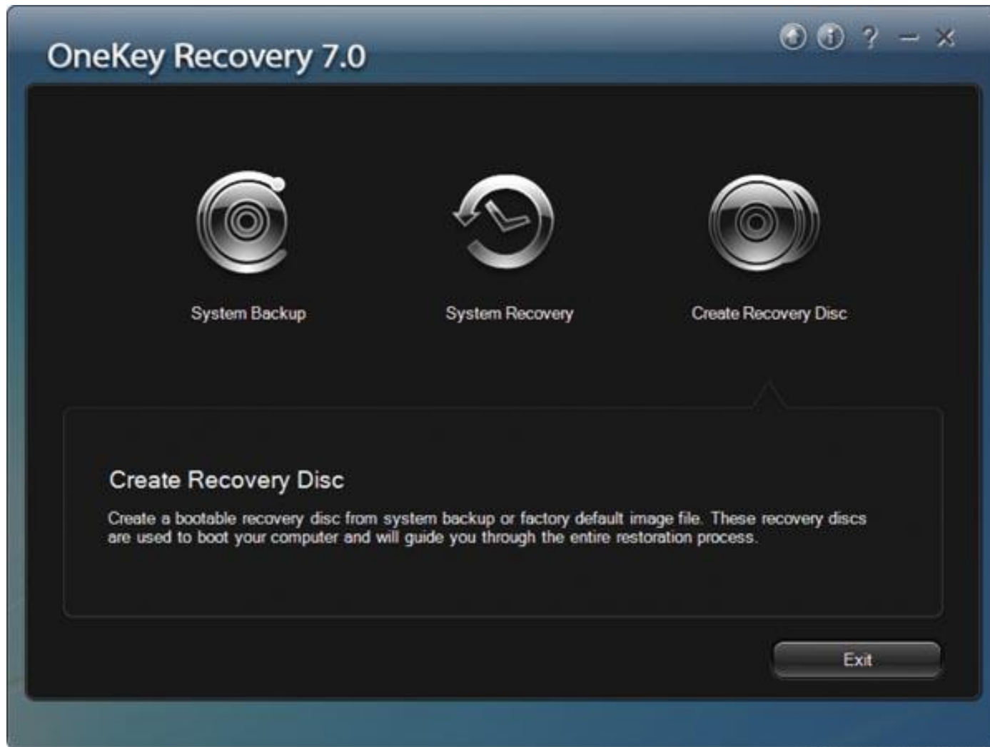
Figure 7-7 Use the recovery utility on this laptop to create DVDs that can be used to recover the system in the event the hard drive fails
